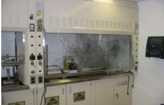
This fume hood sash protected the user because it was down when the event happened.
