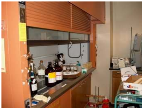
Cluttered hood such as these increase the likelihood of leakage, accident and the severity
